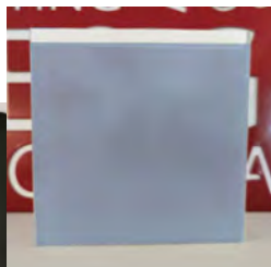
8. PRIVACY SCREEN & MECH. ENCLOSURE- LAMINATED BLUE TINTED SAFETY GLASS WITH FROSTING EFFECT
