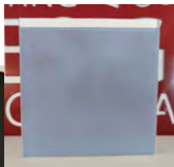
8. PRIVACY SCREEN & MECH. ENCLOSURE- LAMINATED BLUE TINTED SAFETY GLASS WITH FROSTING EFFECT
