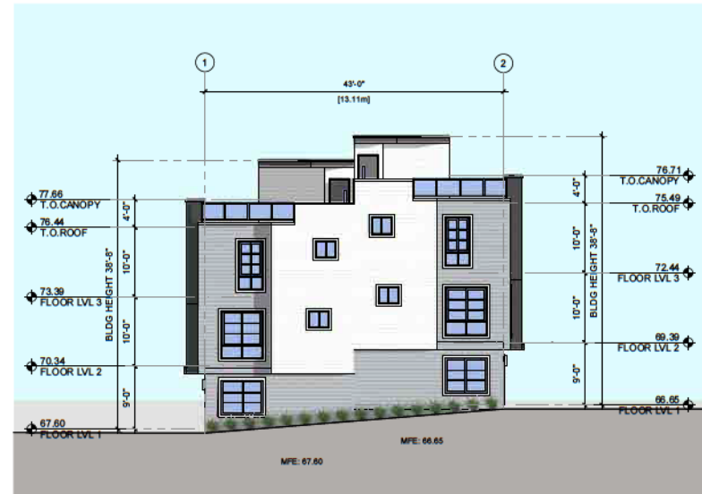
4 BUILDING 6 - WEST ELEVATION SCALE: 1/16" = 1'-0"
