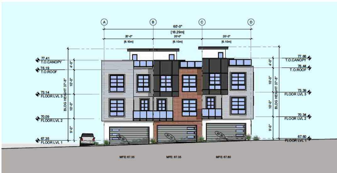
3 BUILDING 3 - SOUTH ELEVATION SCALE: 1/16" = 1'-0"
