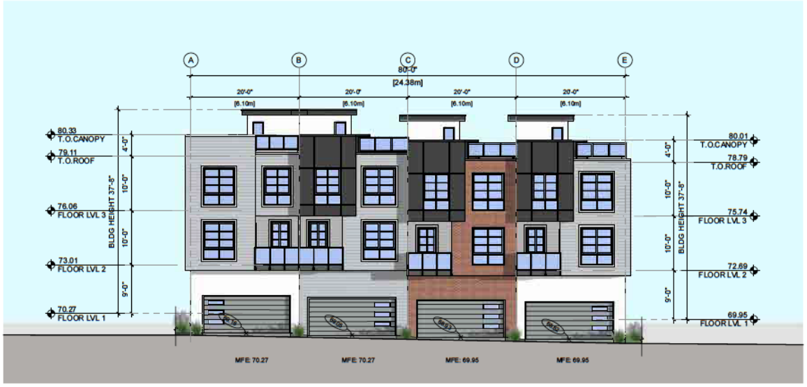
3 BUILDING 7 - NORTH ELEVATION SCALE: 1/16" = 1'-0"
