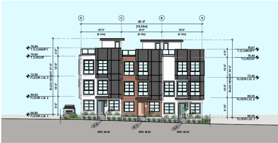
1 BUILDING 4 - NORTH ELEVATION SCALE: 1/16" = 1'-0"
