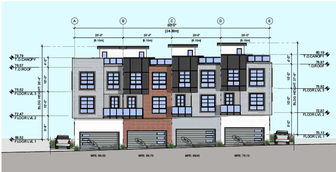
3 BUILDING 2- WEST ELEVATION SCALE: 1/16" = 1'-0"
