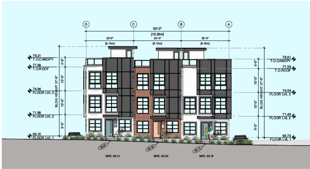
1 BUILDING 1- EAST ELEVATION SCALE: 1/16" = 1'-0"
