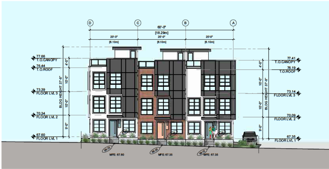
1 BUILDING 3 - NORTH ELEVATION SCALE: 1/16" = 1'-0"
