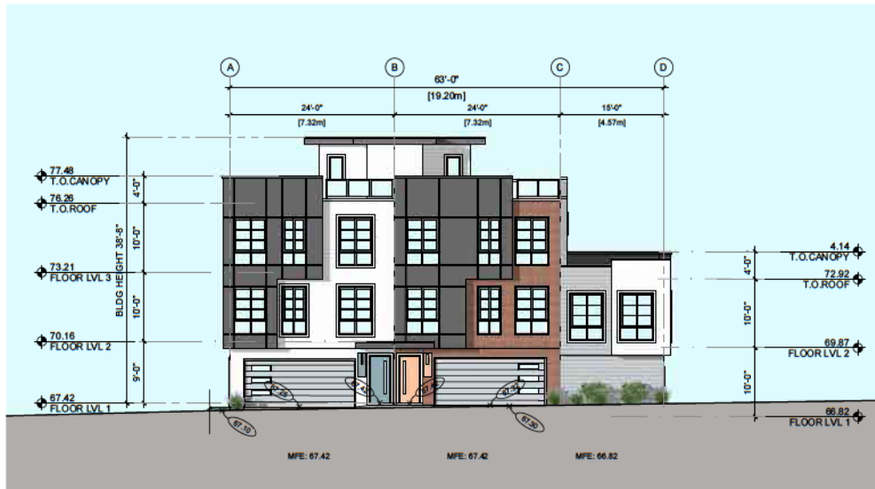
3 BUILDING 5 - SOUTH ELEVATION SCALE: 1/16" = 1'-0"
