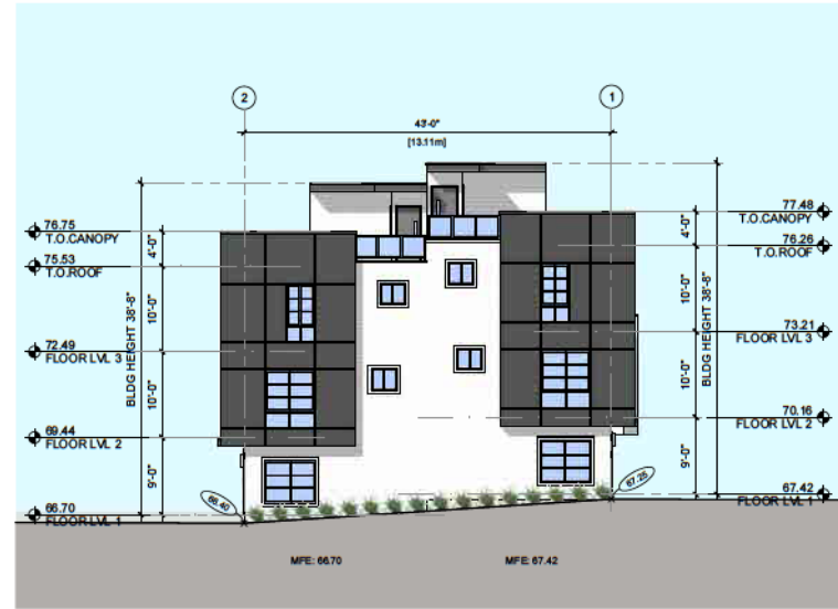
2 BUILDING 5 - WEST ELEVATION SCALE: 1/16" = 1'-0"
