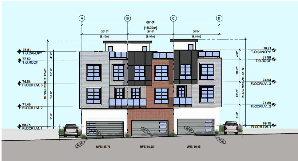
3 BUILDING 1- WEST ELEVATION SCALE: 1/16" = 1'-0"
