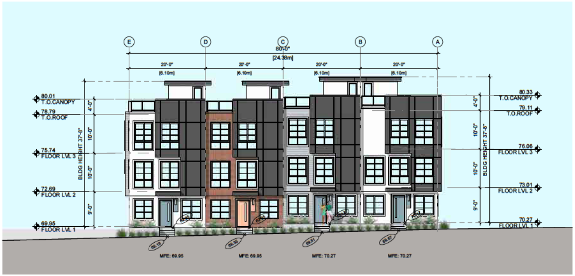
1 BUILDING 7 - SOUTH ELEVATION SCALE: 1/16" = 1'-0"
