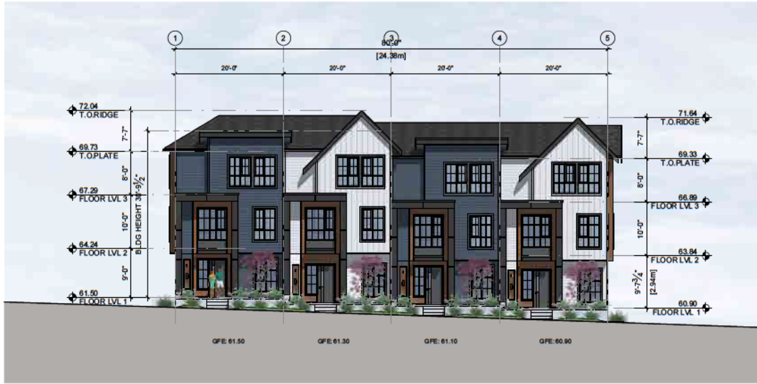
1 BUILDING3- EAST ELEVATION SCALE: 1/16" = 1'-0"
