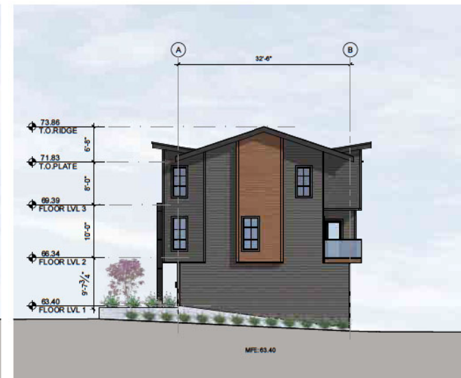
4 BUILDING4- NORTH ELEVATION SCALE: 1/16" = 1'-0"
