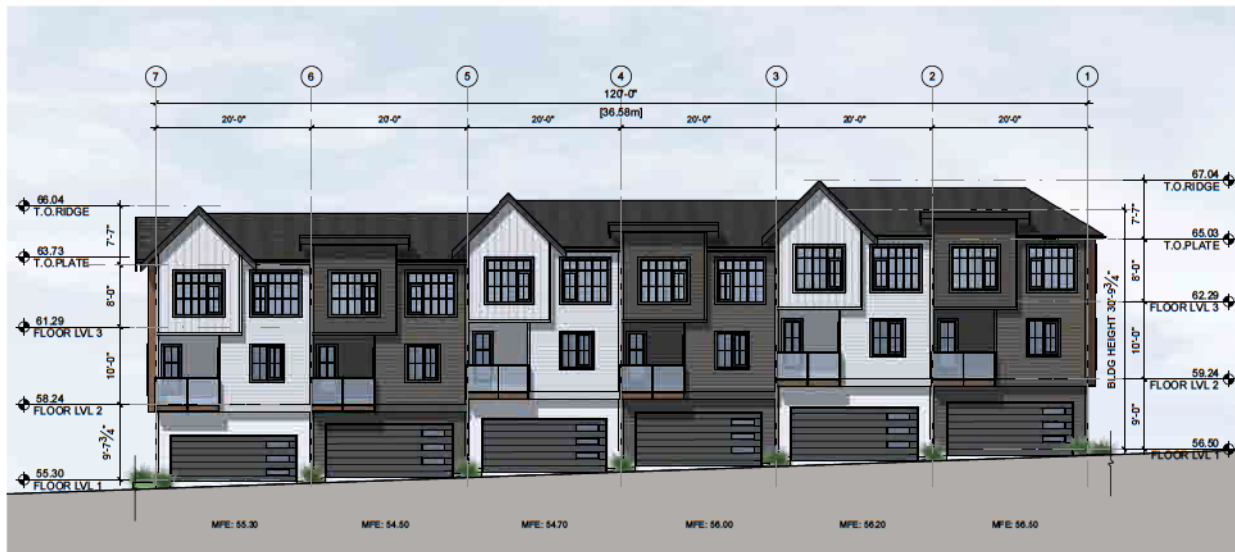
3 BUILDING13- SOUTH ELEVATION SCALE: 1/16" = 1'-0"
