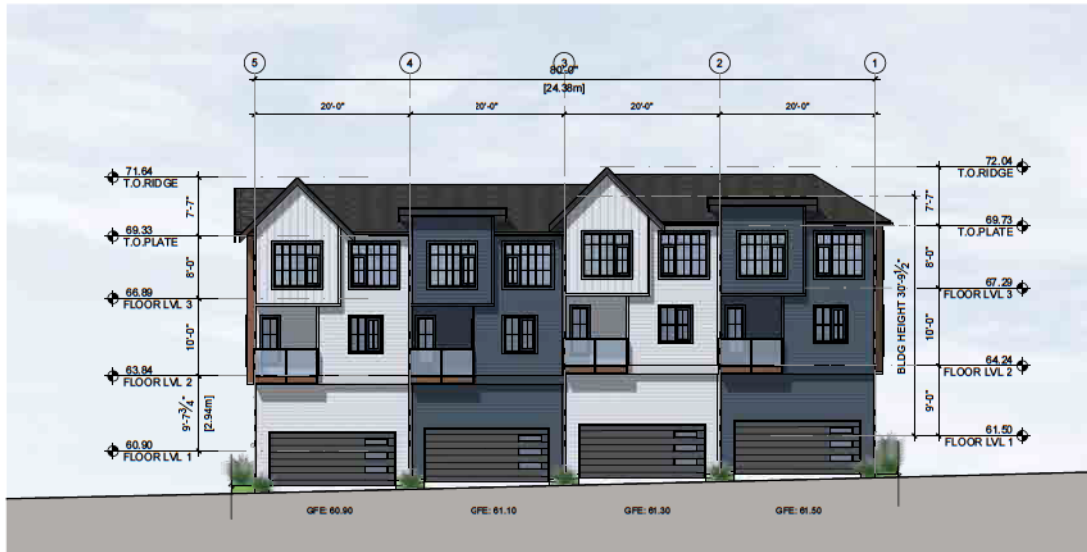
3 BUILDING3- WEST ELEVATION SCALE: 1/16" = 1'-0"
