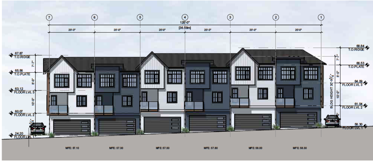
3 BUILDING1- SOUTH ELEVATION SCALE: 1/16" = 1'-0"
