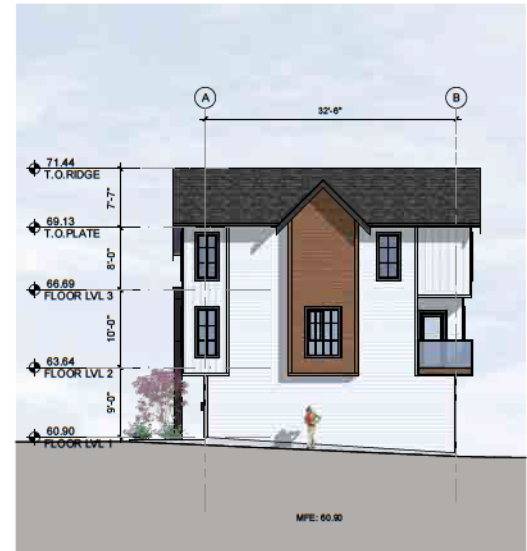
4 BUILDING3- EAST ELEVATION SCALE: 1/16" = 1'-0"
