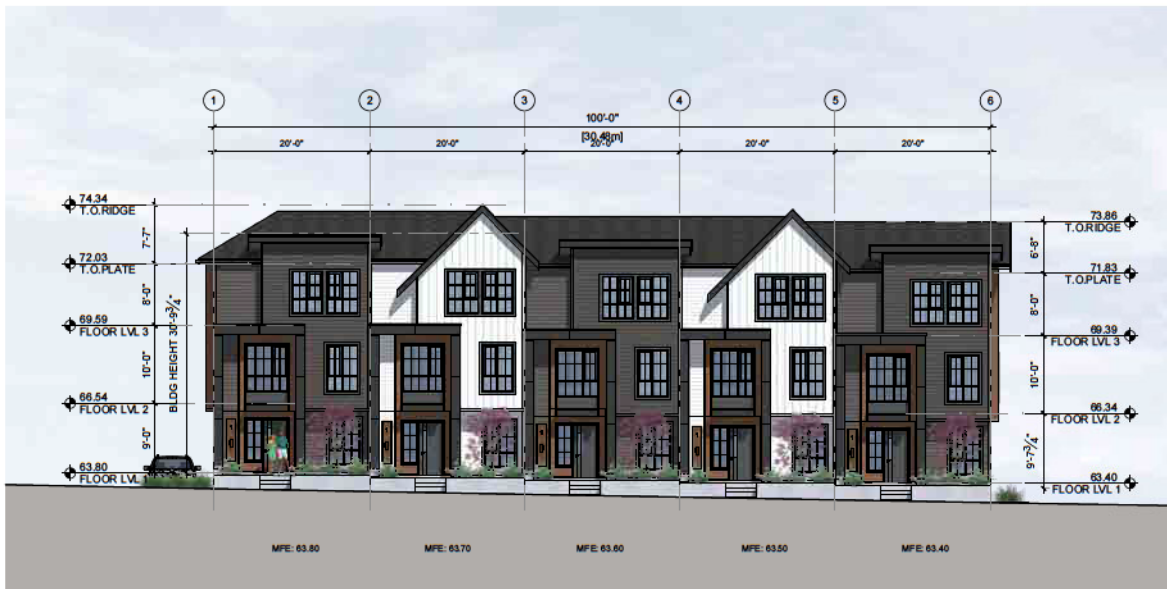
1 BUILDING4- EAST ELEVATION SCALE: 1/16" = 1'-0"
