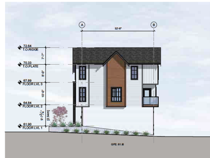
4 BUILDING4- NORTH ELEVATION SCALE: 1/16" = 1'-0"
