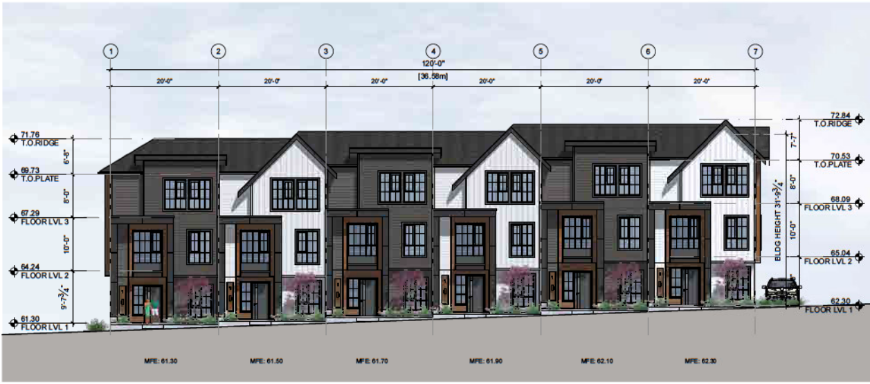
1 BUILDING2- SOUTH ELEVATION SCALE: 1/16" = 1'-0"
