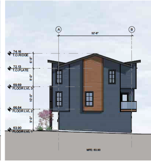
4 BUILDING1- EAST ELEVATION SCALE: 1/16" = 1'-0"
