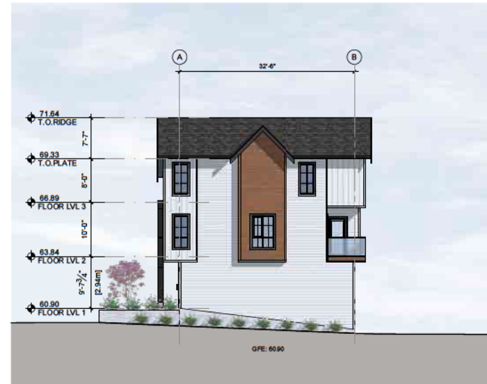
4 BUILDING3- NORTH ELEVATION SCALE: 1/16" = 1'-0"
