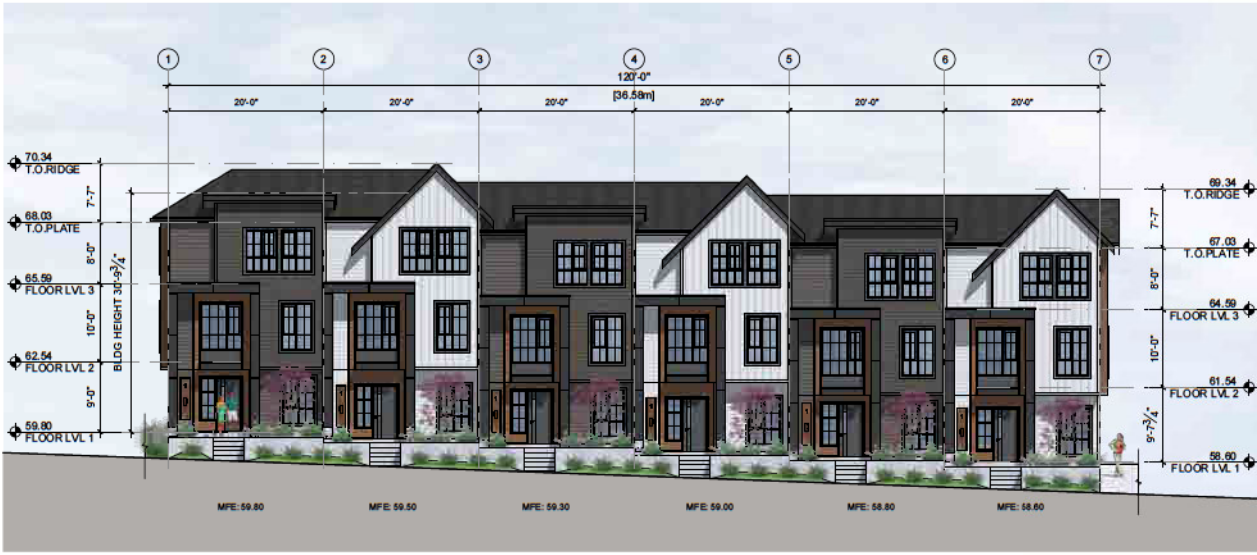
1 BUILDING2- NORTH ELEVATION SCALE: 1/16" = 1'-0"
