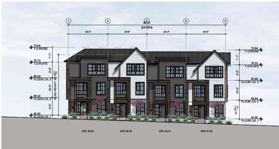
1 BUILDING4- EAST ELEVATION SCALE: 1/16" = 1'-0"
