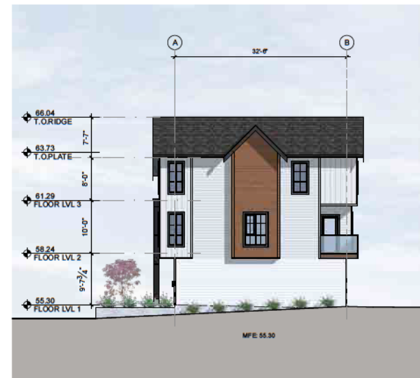
4 BUILDING13- WEST ELEVATION SCALE: 1/16" = 1'-0"
