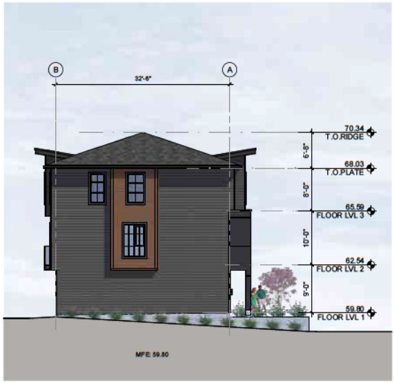
2 BUILDING2- EAST ELEVATION SCALE: 1/16" = 1'-0"
