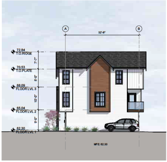
4 BUILDING2- EAST ELEVATION SCALE: 1/16" = 1'-0"
