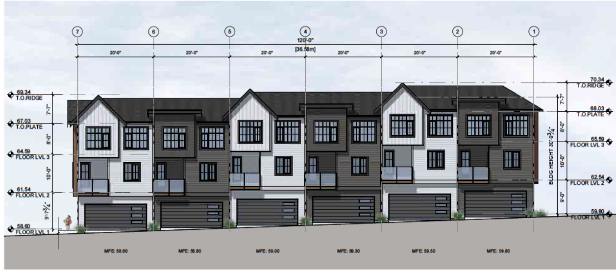
3 BUILDING2- SOUTH ELEVATION SCALE: 1/16" = 1'-0"
