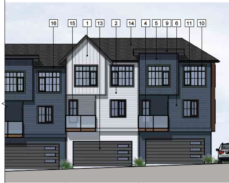
2 BLDG 1 - SOUTH ELEVATION SCALE: 3/32 = 1'-0"
